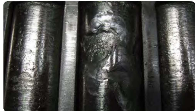
Damaged outer taper roller bearing
